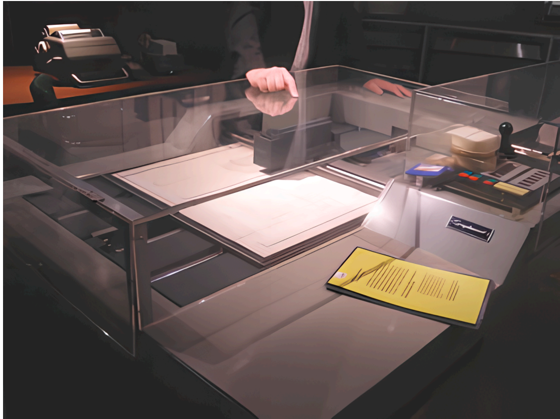
Figure 2.2: Image of the Zuse Graphomat Z64 plotter, a versatile device originally designed for technical drawing and other industrial applications. However, some artists and designers repurposed the plotter for creating generative art, a style of art that relies on algorithms and mathematical formulas to generate complex patterns and designs.
